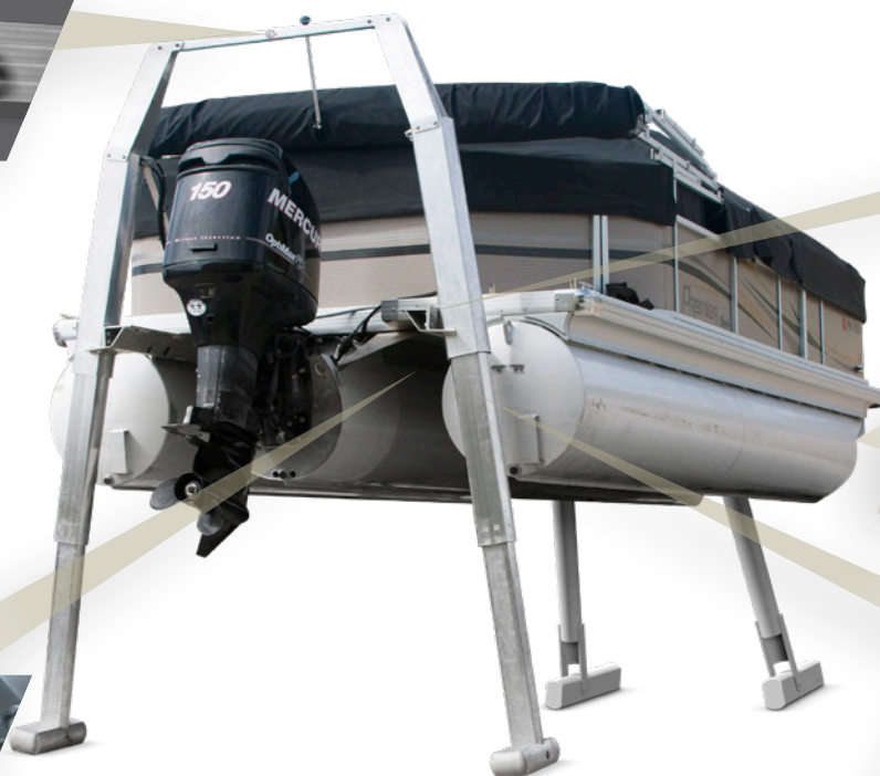
REAR LEG PLACEMENT IN RETRACTED POSITION
