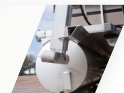
REAR LEG PLACEMENT IN RETRACTED POSITION
