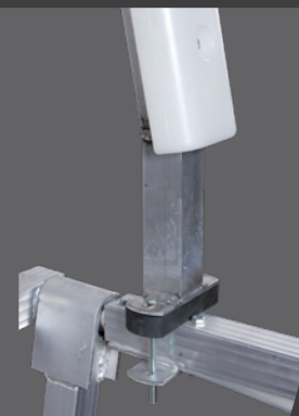
RUBBER MOUNTED CENTERING GUIDES
